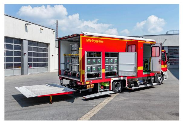
ZIEGLER recently delivered a new vehicle to the fire department of Lünen. The vehicle is equipped with numerous advanced features: for example, it offers separate interior compartments in the black and white area for clean and contaminated materials, which enables effective decontamination and cleaning. The loading area offers space for up to six roll containers so that a wide range of equipment can be transported safely.
