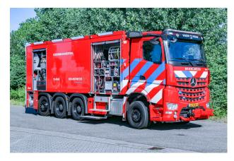
firefighting. The two remote-controlled front and roof turrets deliver the extinguishing agent safely and accurately. The vehicle is also equipped with a 250 kg powder extinguishing system.
