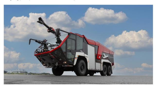
The vehicle was built on a TITAN 6x6 chassis T39-770 6x6 and is equipped with a 770 HP Scania V8 engine. The engine with Stage V emission level exceeds the current emission regulations by far. The innovative and stepless transmission by Kessler completes the driveline concept and brings this high performance actually on the road. As a result, the vehicle achieves acceleration values from 0 to 80 km/h in less than 30 seconds.
