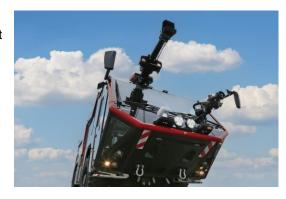
The driver's cab (Z-Cab AiR) is certified according to crash test ECE R 29-3 and thus offers the best possible crew protection. The vehicle can be handled and controlled using the latest generation of the intuitive Z-Control operating concept.
