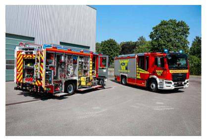
Based on an MAN TGM 15.290 chassis with a wheelbase of 4,125 mm, the two HLF 20 have an output of 213 kW / 290 HP while complying with the EURO 6 emissions standard. The permissible gross weight is 15,500 kg. This makes extensive equipment or loading possible.
